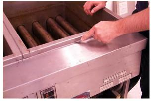
Cutting frypot seal prior to frypot removal.
